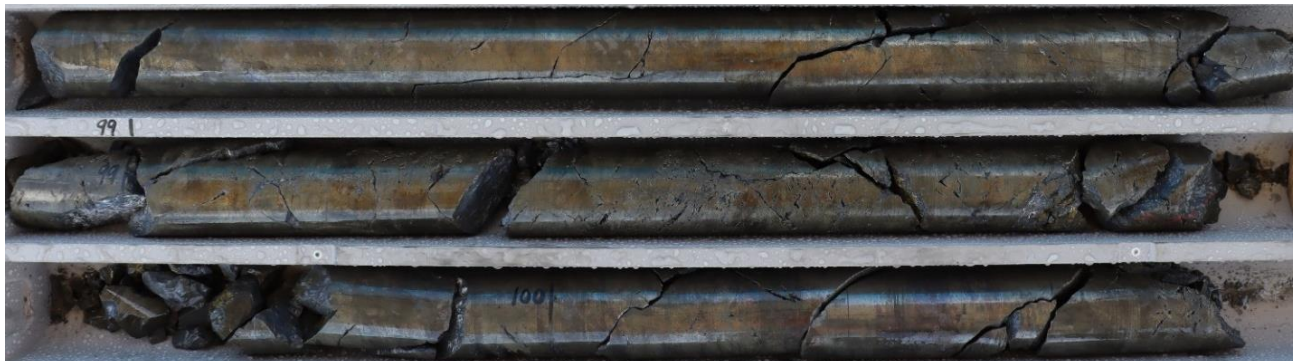
Figure 1. 22DMDD009 1 98.95-101.5m Massive pyrite chalcocite with minor relict chalcopyrite, bornite and sphalerite.
