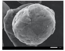
Scanning electron microscopy of high purity alumina doped coated spherical graphite
