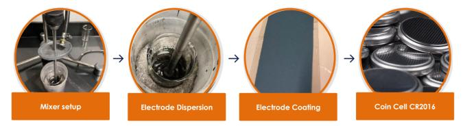
Electrochemical performance of the coated spherical graphite (coated anode) and FYI HPA-doped coated spherical graphite HPA-doped coated anode) was undertaken in an industry standard lithium-ion coin cell (CR2016).
