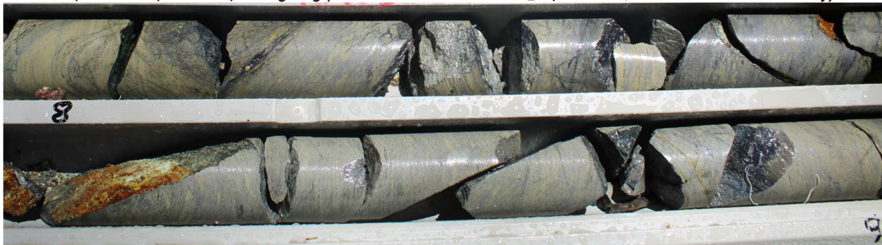
Figure 2: Part of Core from 8–9.0m downhole showing high grade massive sulphide mineralisation that includes portions of the 1m interval from 7.7-8.7m @ 43.30% Zn, 17.50% Pb, 3.06% Cu, 73.20g/t Ag and the upper 0.3m of the 0.9m from 8.7-9.7m @ 42.30% Zn, 16.45% Pb, 1.88% Cu, 51.90g/t Ag (Diamond drill hole CRRDD21_06, Scale: NQ core 50mm diameter variety)
