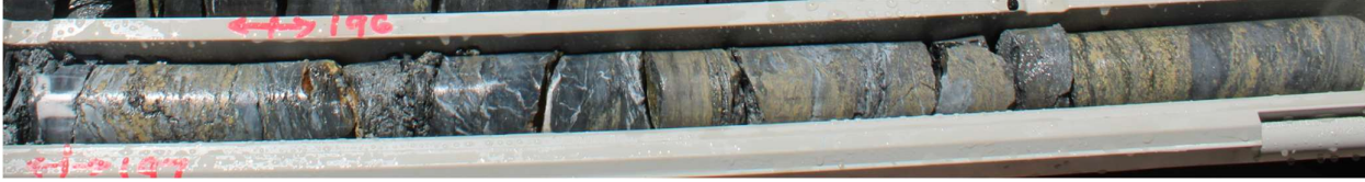
Figure 5: Massive sulphide mineralisation, detail of core from Figure 4 (RHS 8.7-9m), the mineralisation is dominated by yellow-brown, low iron sphalerite (Zinc Sulphide) (Diamond drill hole CRRDD21_05, Scale: NQ core 50mm diameter variety)
