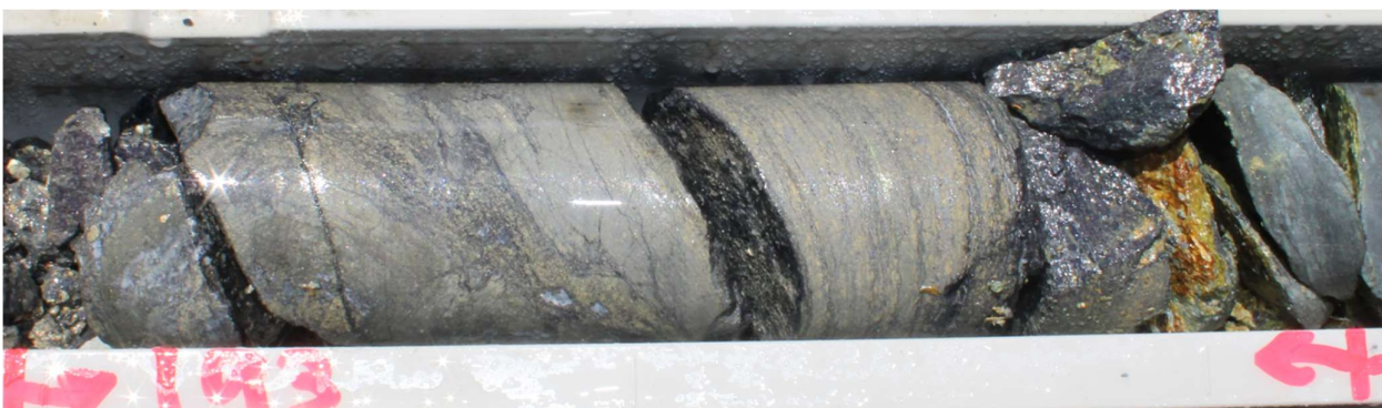
Figure 6: Shallow massive sulphide mineralisation, core from 5.69-5.91m downhole that assayed 26.40% Zn, 15.55% Pb, 6.11% Cu, 56.60g/t Ag (Diamond drill hole CRRDD21_05, Scale: NQ core 50mm diameter variety)
