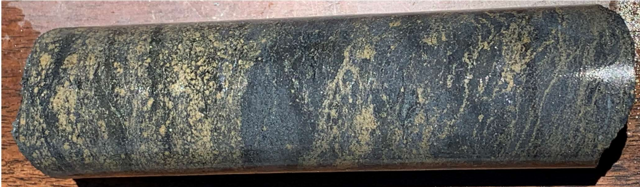
Figure 6: Shallow massive sulphide mineralisation, core from 5.69-5.91m downhole that assayed 26.40% Zn, 15.55% Pb, 6.11% Cu, 56.60g/t Ag (Diamond drill hole CRRDD21_05, Scale: NQ core 50mm diameter variety)
