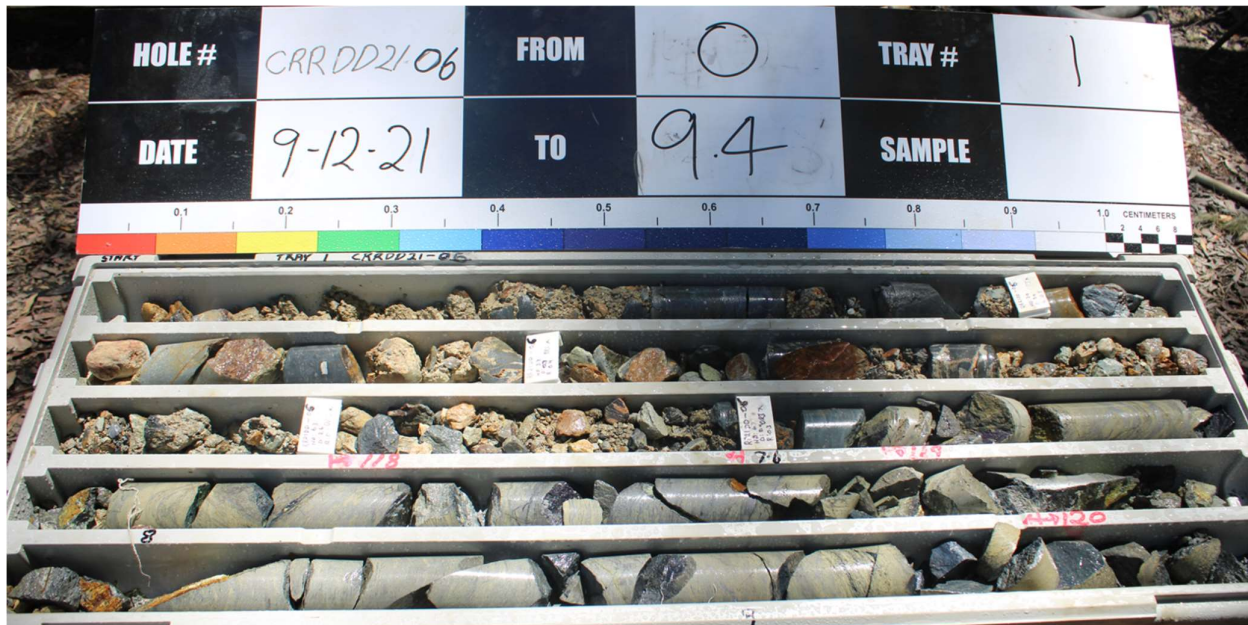
Figure 2: Part of Core from 8–9.0m downhole showing high grade massive sulphide mineralisation that includes portions of the 1m interval from 7.7-8.7m @ 43.30% Zn, 17.50% Pb, 3.06% Cu, 73.20g/t Ag and the upper 0.3m of the 0.9m from 8.7-9.7m @ 42.30% Zn, 16.45% Pb, 1.88% Cu, 51.90g/t Ag (Diamond drill hole CRRDD21_06, Scale: NQ core 50mm diameter variety)
