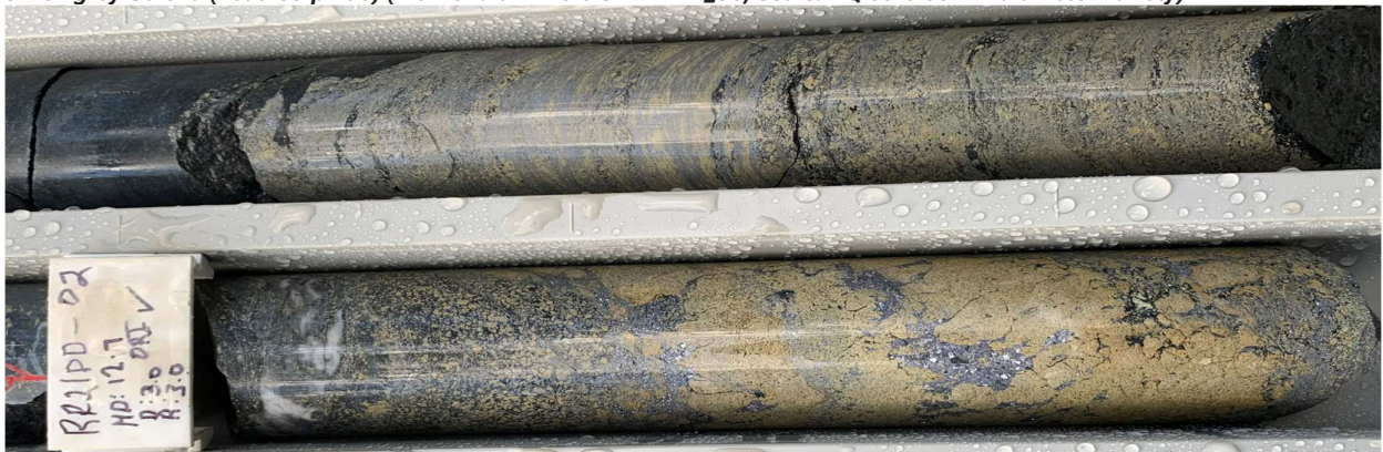
Figure 3: Massive sulphide mineralisation, the lower row shows core from 12.67–13.0m downhole that assayed 31.30% Zn, 20.90% Pb, 0.97% Cu, 96.0g/t Ag. The mineralisation is dominated by yellow-brown, low iron sphalerite (Zinc Sulphide) and silver-grey Galena (Lead Sulphide) (Diamond drill hole CRRDD21_06, Scale: NQ core 50mm diameter variety)
