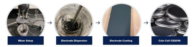
Electrochemical performance of the coated spherical graphite (coated anode) and HPA-doped coated spherical graphite (HPA-doped coated anode) was undertaken in an industry standard coin cell (CR2016) to determine the performance in a lithium-ion cell which are used to power EV's.
