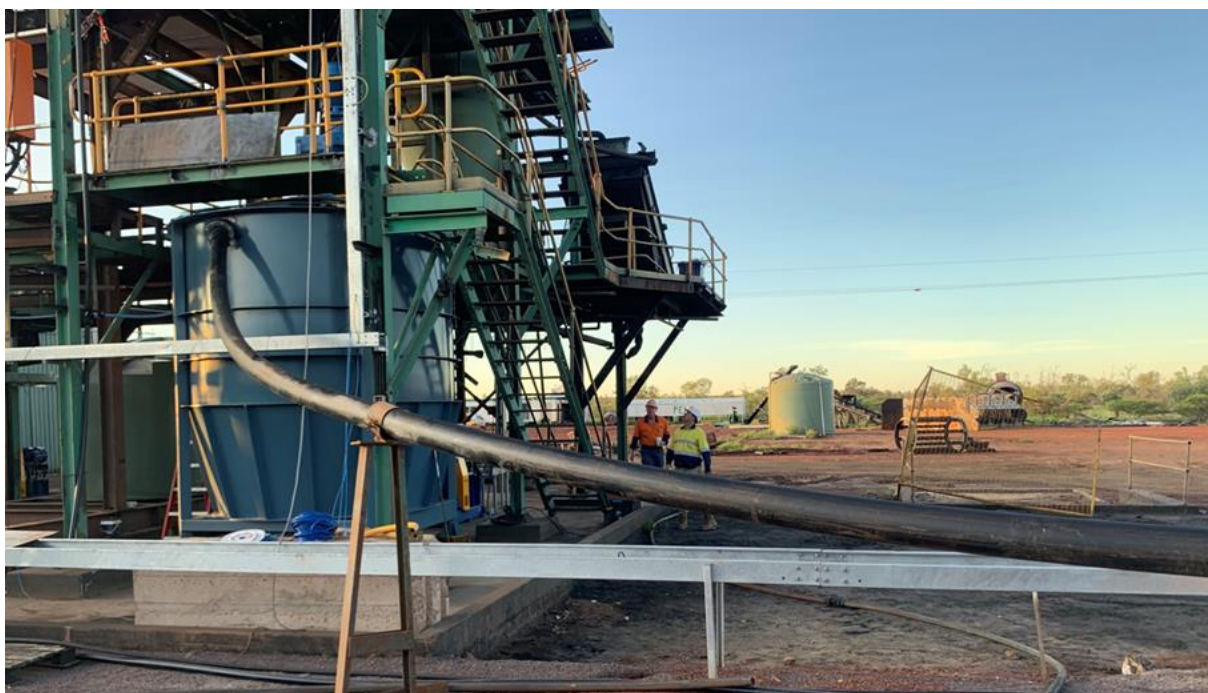
Main feed from scrubber to mixing and magnetic separation tower
