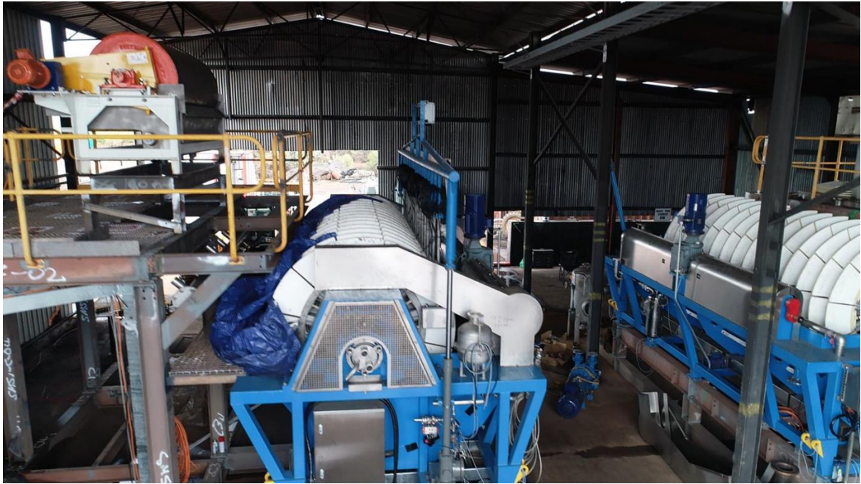
Twin ceramic disk filters and magnetic separators for drying final product.
