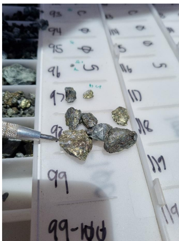
Figure 4: Visible Chalcopyrite (copper sulphide) in Drill Chips from Hole 22GTRCOO5
