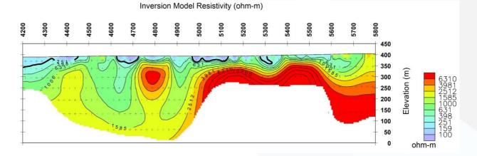
Figure 7. IP line L18600N Inversion Model Resistivity Section.
