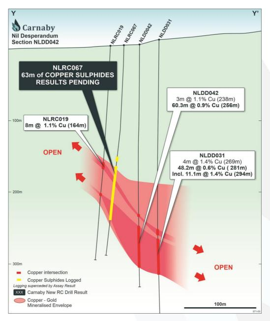
Figure 4. Drill Section showing location of drill hole NLRC067.
