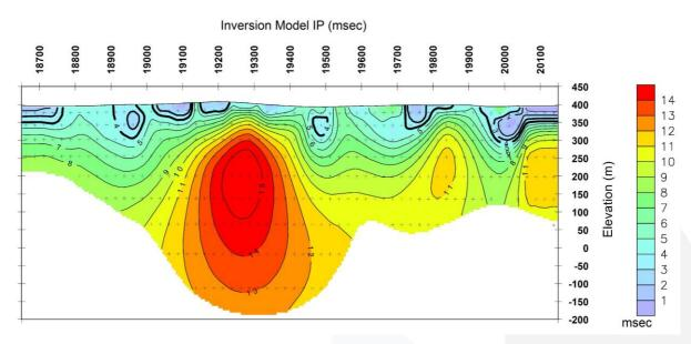
Figure 6. IP line L4900E Inversion Model Chargeability Section.
