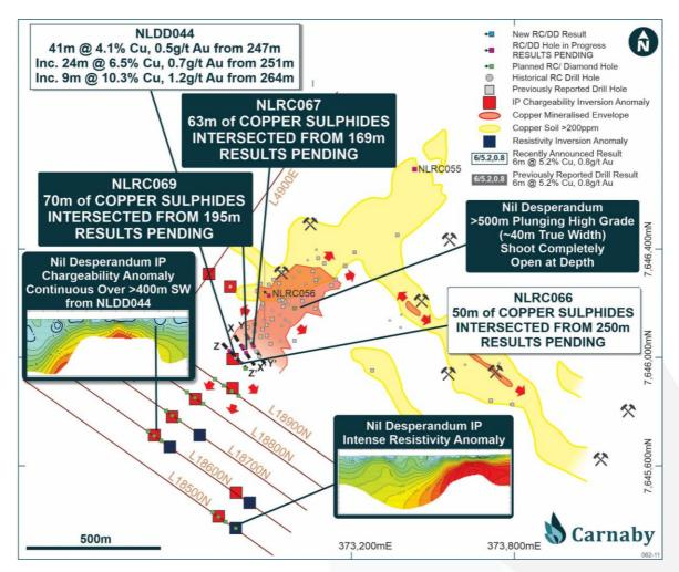
Figure 1. Plan of Nil Desperandum Showing location of NLRC067, NLRC069 and IP.
