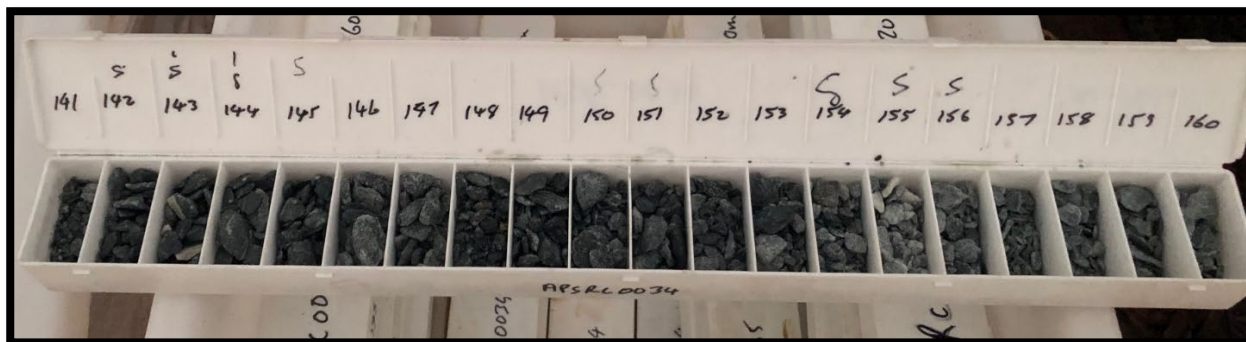
Photo 2: Chip tray from hole APSRC0034 depth 140-160m showing sulphides in a basaltic (140-145) and gabbro (145-156) units
