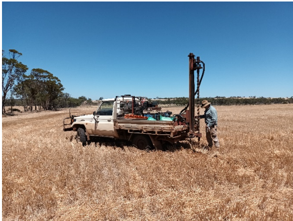
Figure 2: Auger drilling underway, Calingiri East
