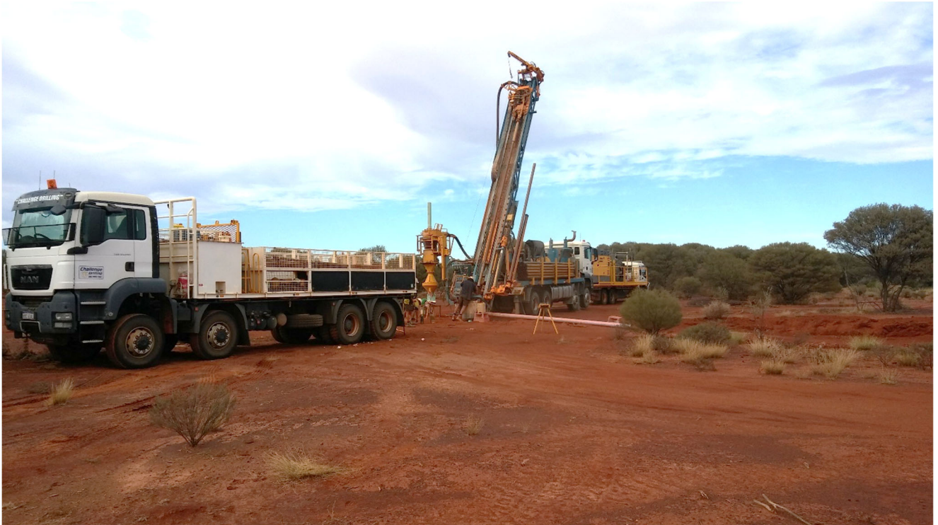
Figure 4: RC drilling at Indomitabile
