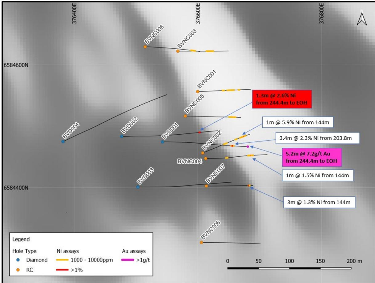
**Figure 3.** Commodore drill plan over airborne magnetics showing RC and Diamond Drilling. New results shown in bold (*magenta = gold, red = nickel*)
