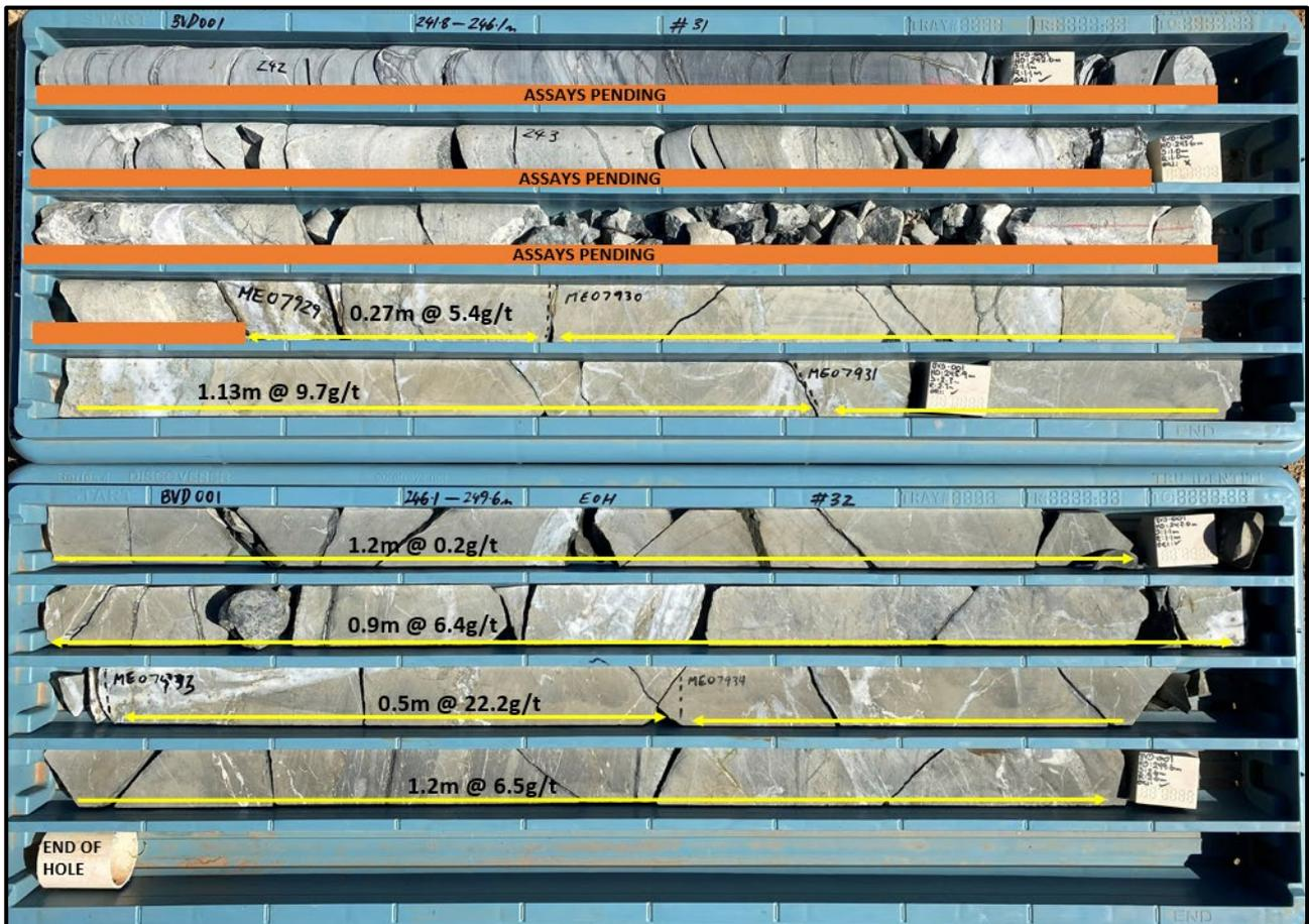
**Figure 2.** Mineralised drillcore from BVD001 showing gold intersections
