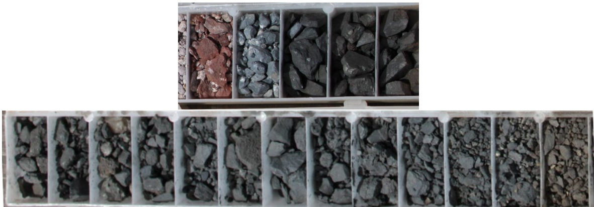
Image 2 / RC drill chips: 21MDRC011, 56-73m (17m @ 0.84% Cu & 462ppm Co, chalcocite & covellite mineralisation)
