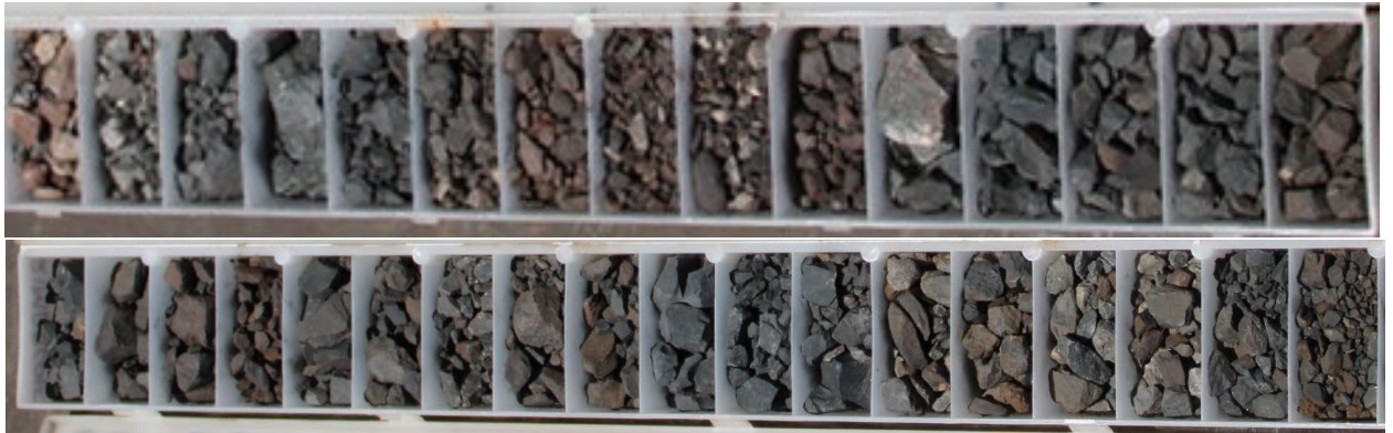
Image 4 / RC drill chips: 21MDRC015 65-76m (11m @ 2.27% Cu & 429ppm Co & 78-98m 20m @ 1.99% Cu & 30ppm Co, chalcocite & covellite mineralisation)
