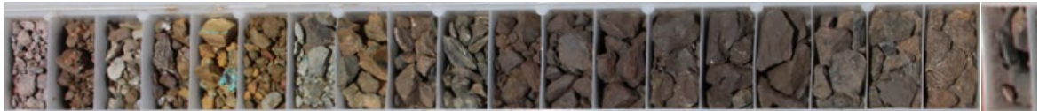
Image 5 / RC drill chips: 21MDRC016 41-61m (20m @ 0.86% Cu & 609ppm Co malachite, cuprite & chalcocite mineralisation)
