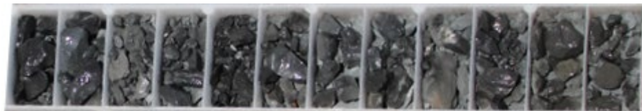
Image 7 / RC drill chips: 21MDRC018 108-117m (9m @ 0.95% Cu & 284ppm Co. pyrite & chalcopyrite mineralisation)
