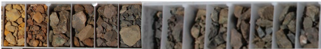
Image 8 / RC drill chips: 21MDWB02 34-48m (14m @ 0.81% Cu & 366ppm Co. malachite & cuprite mineralisation)
