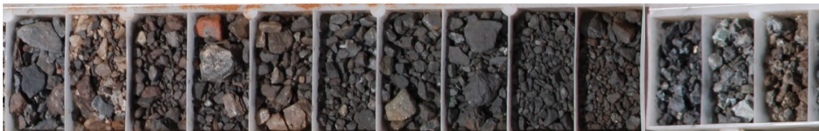
Image 3 / RC drill chips: 21MDRC012, 50-63m (13m @ 0.85% Cu & 429ppm Co, cuprite, chalcocite & covellite mineralisation)
