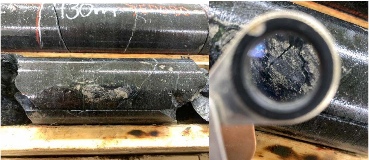
Figure 2: DDED22-080 coarse pentlandite-pyrrhotite intergrowth at 431.4m
