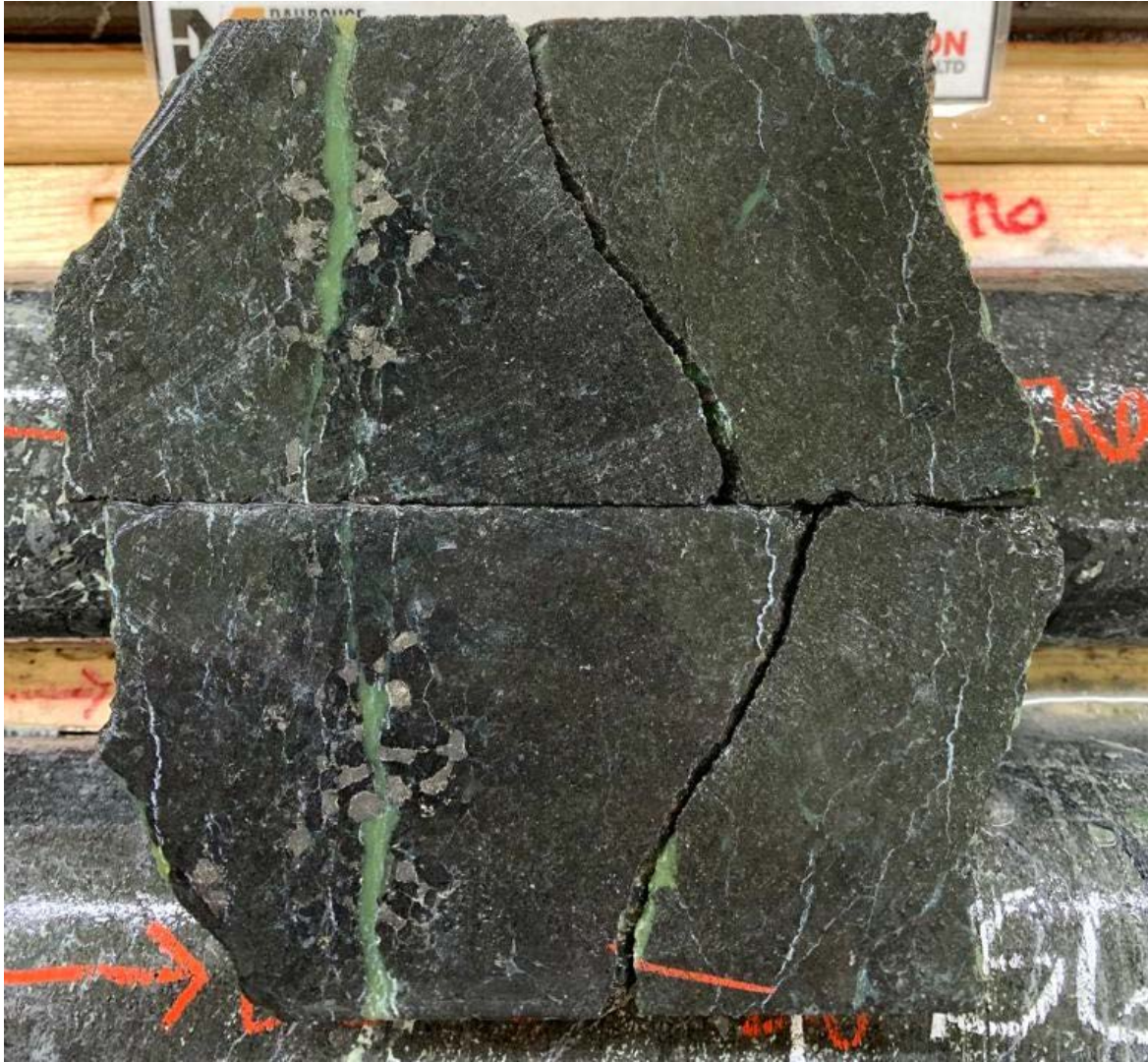
Figure 9: DDED22-080 blebby pentlandite-pyrrhotite mineralisation at 488m
