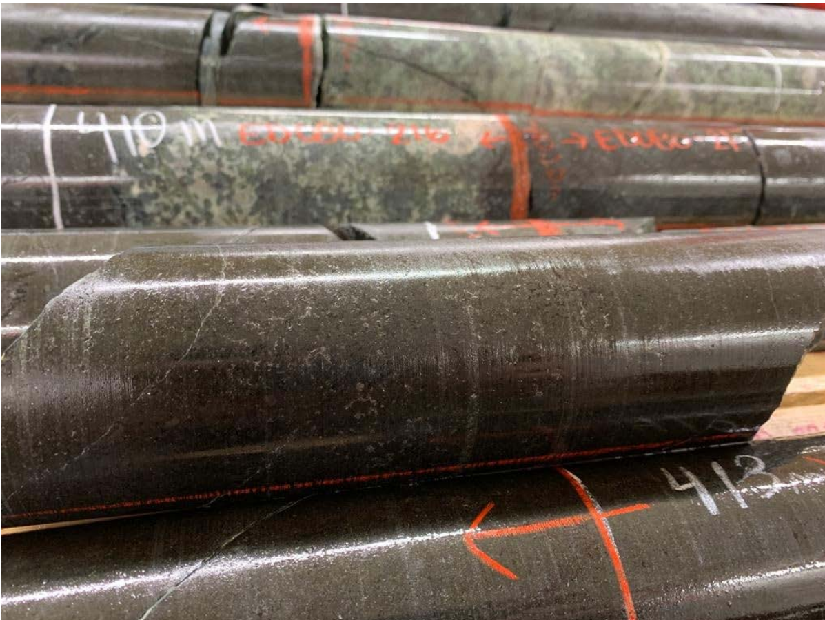
Figure 6: DDED22-080 disseminated pentlandite-pyrrhotite mineralisation at 412m
