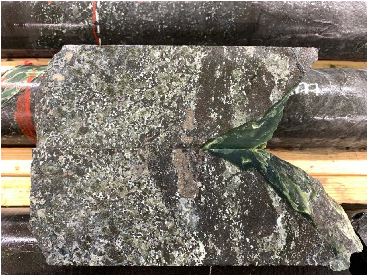
Figure 8: DDED22-080 blebby pentlandite-pyrrhotite mineralisation at 455.7m
