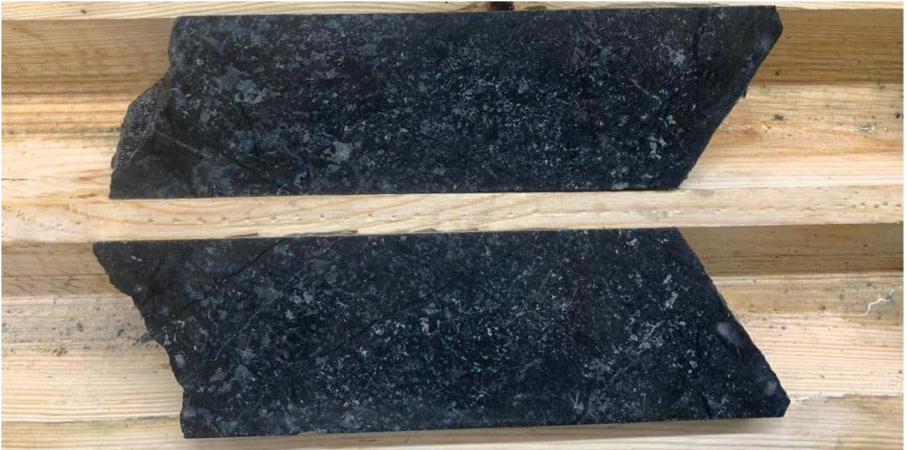
Figure 7: DDED22-080 disseminated pentlandite-pyrrhotite mineralisation at 420m
