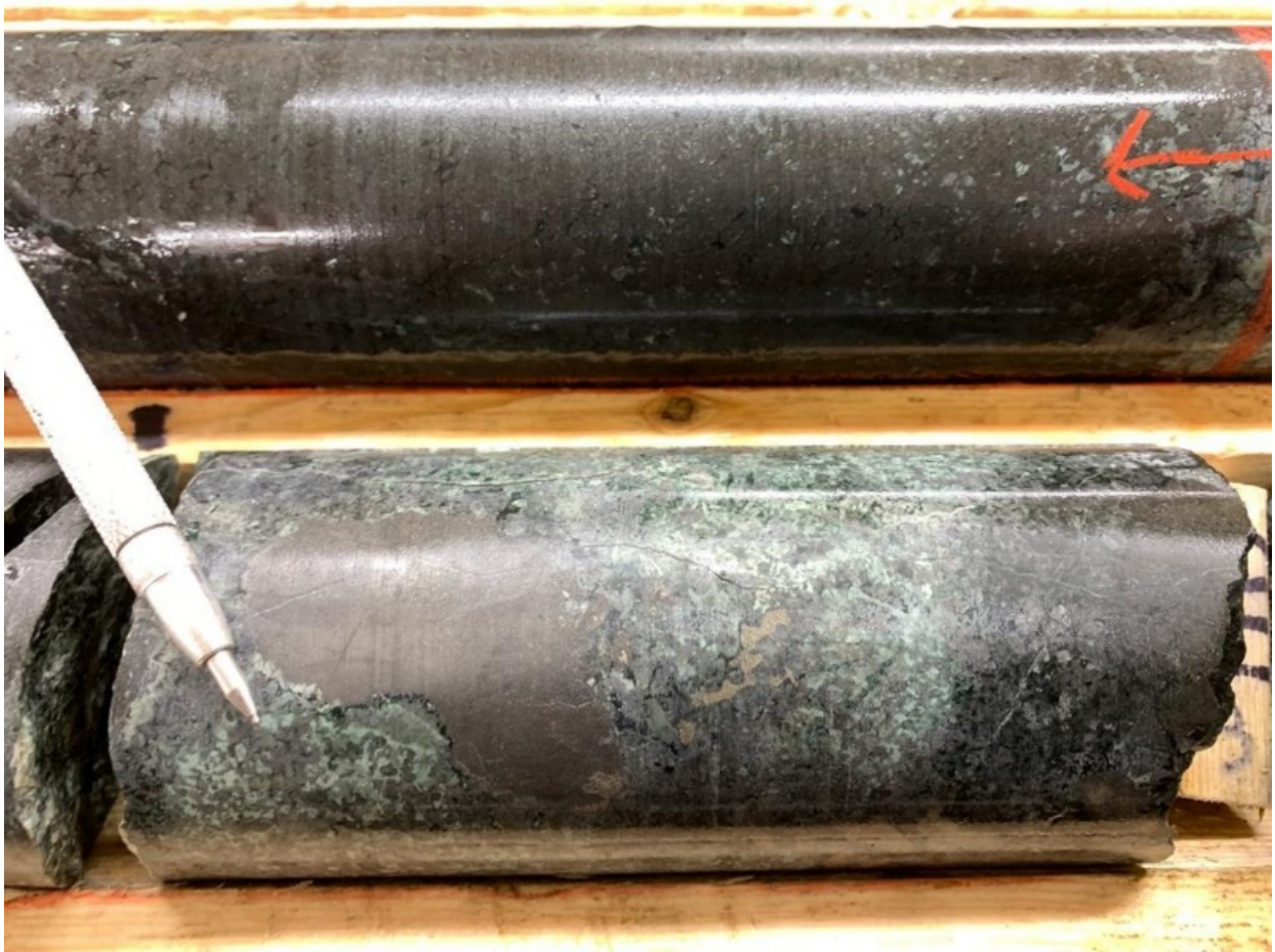
Figure 1: DDED22-080 clast of semi-massive pentlandite-pyrrhotite with blebby to disseminated pentlandite-pyrrhotite at 411.2m
