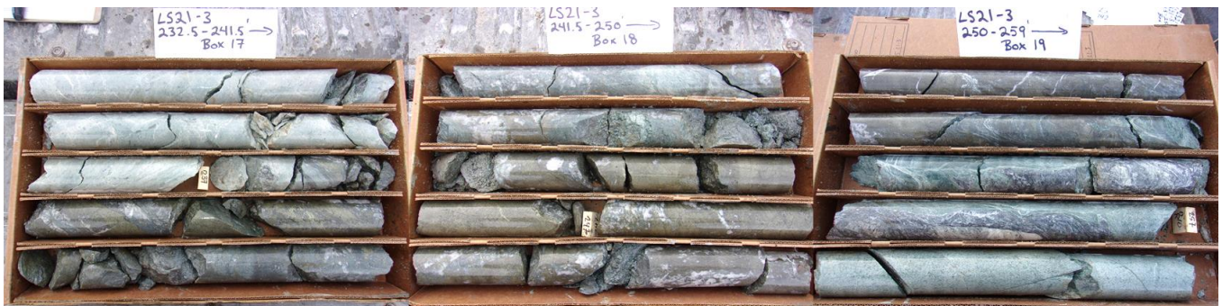
Figure 1: Drill hole LS21-003 from 70.87m (232.5ft) – 78.94m (259ft), core blocks represent downhole depth in feet, highlighting observed quartz veins with massive sulphide.
