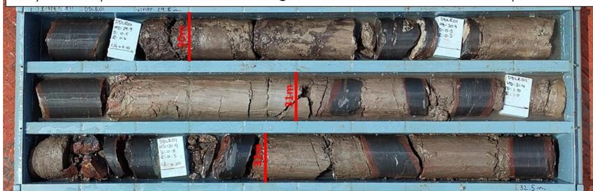
Assay result from previous twinned hole LRRC08 - 3m @ 15.3% Mn & 10.5% Fe from 30m over the equivalent interval
