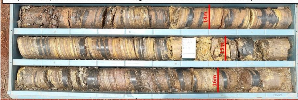
Assay result from previous twinned hole LRRC08 - 3m @ 11.5% Mn & 8.8% Fe from 13m over the equivalent interval
