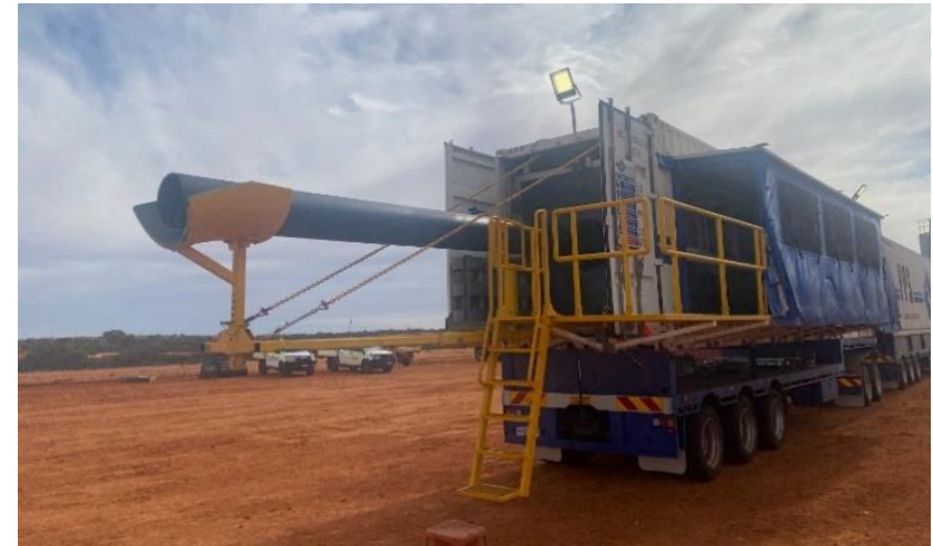
PPS Extruder First HDPE pipe extruded at Ambassador (8 December 2021)
