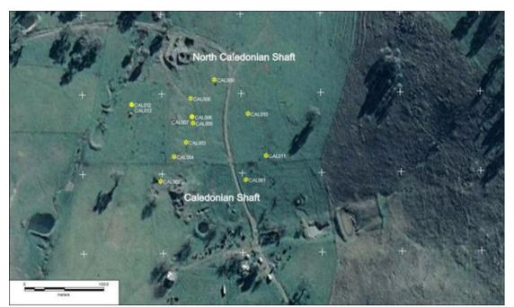
*Figure 1: Position for an initial 13 drill holes which vary depending on drill results*
