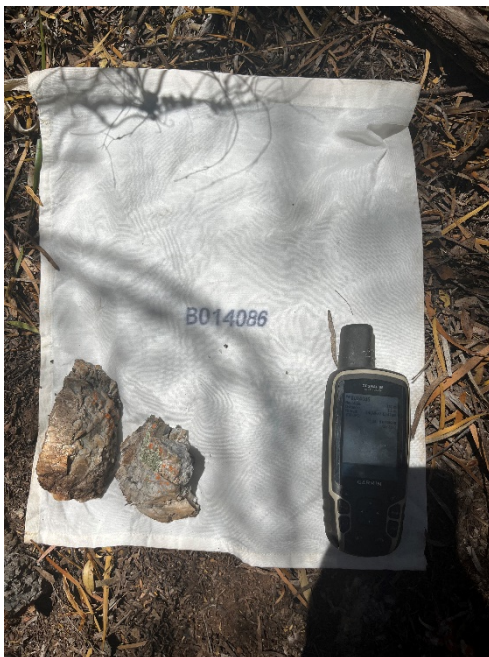
Sample B014086 (Spodumene and quartz) = 3.92 % \text{Li}_2\text{O}
