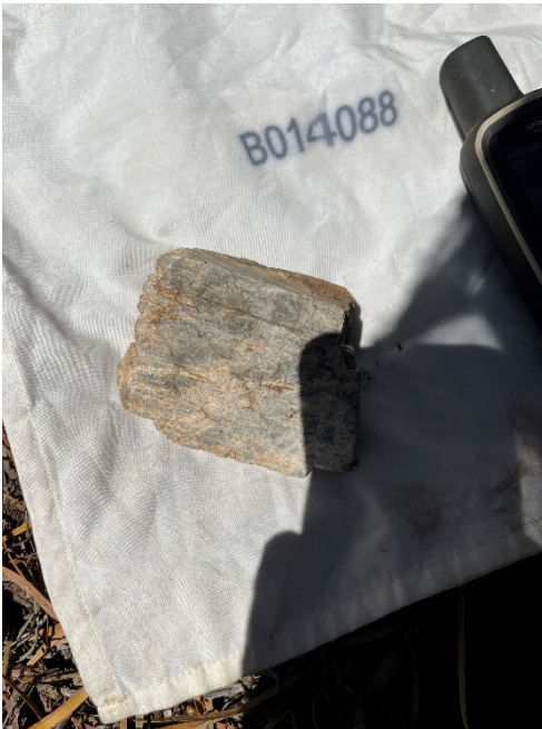
Sample B014088 (Spodumene) = 6.95 % \text{Li}_2\text{O}
