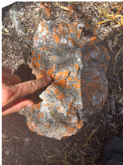
Sample B014086 (Spodumene and quartz) = 3.92 % \text{Li}_2\text{O}
