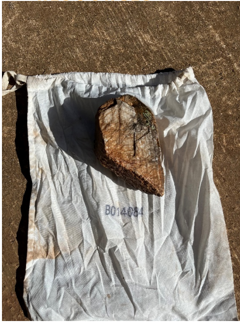
Sample B014084 (Amblygonite) = 8.21 % \text{Li}_2\text{O}
