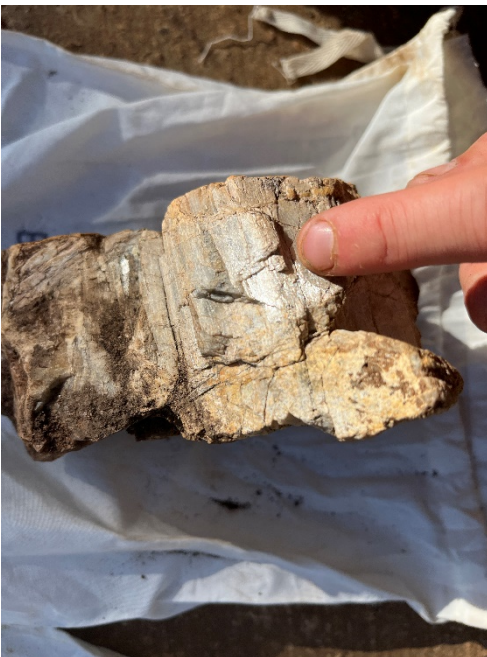
Sample B014083 (Spodumene and quartz) = 5.45 % \text{Li}_2\text{O}
