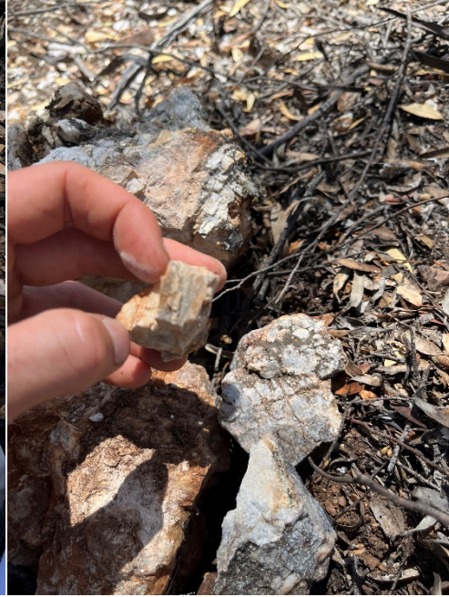
Sample B014087 (Spodumene and quartz) = 3.83 % \text{Li}_2\text{O}
