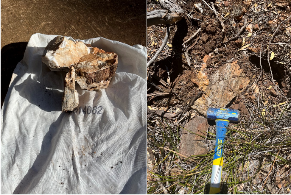
Sample B014082 (Quartz and spodumene) = 4.18 % \text{Li}_2\text{O}
