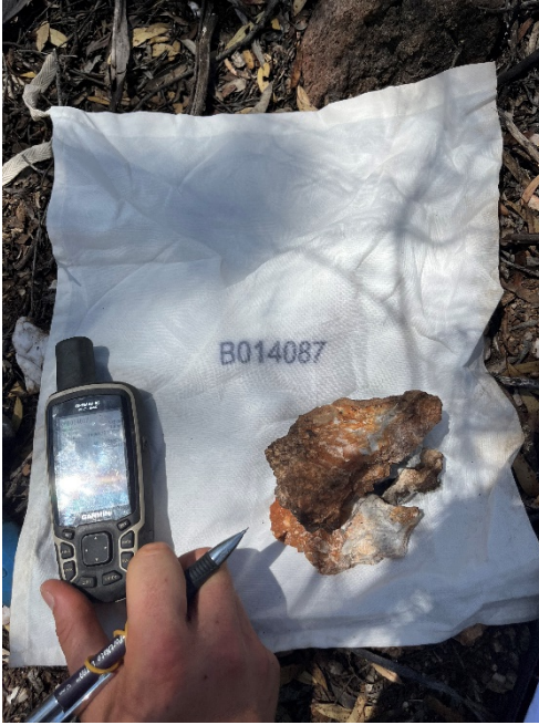
Sample B014087 (Spodumene and quartz) = 3.83 % \text{Li}_2\text{O}
