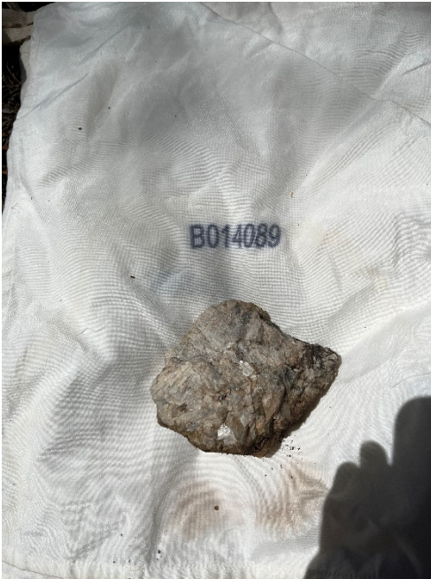
Sample B014089 (Spodumene) = 5.39 % \text{Li}_2\text{O}
