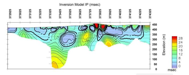
Figure 4. IP line L7649675N chargeability inversion showing location of anomalies.
