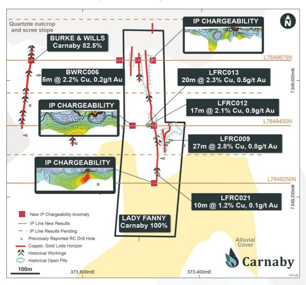
Figure 1. Lady Fanny Plan Showing new IP inversion chargeability anomalies.
