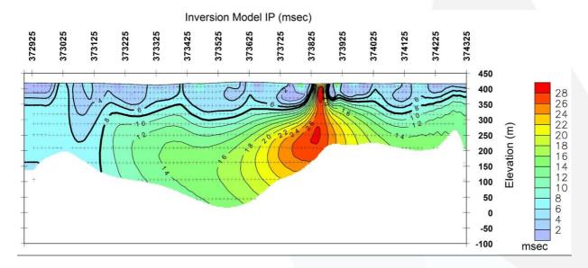
Figure 2. IP line L7649250N chargeability inversion showing location of anomaly.
