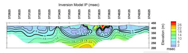
Figure 3. IP line L7649450N chargeability inversion showing location of anomalies.
