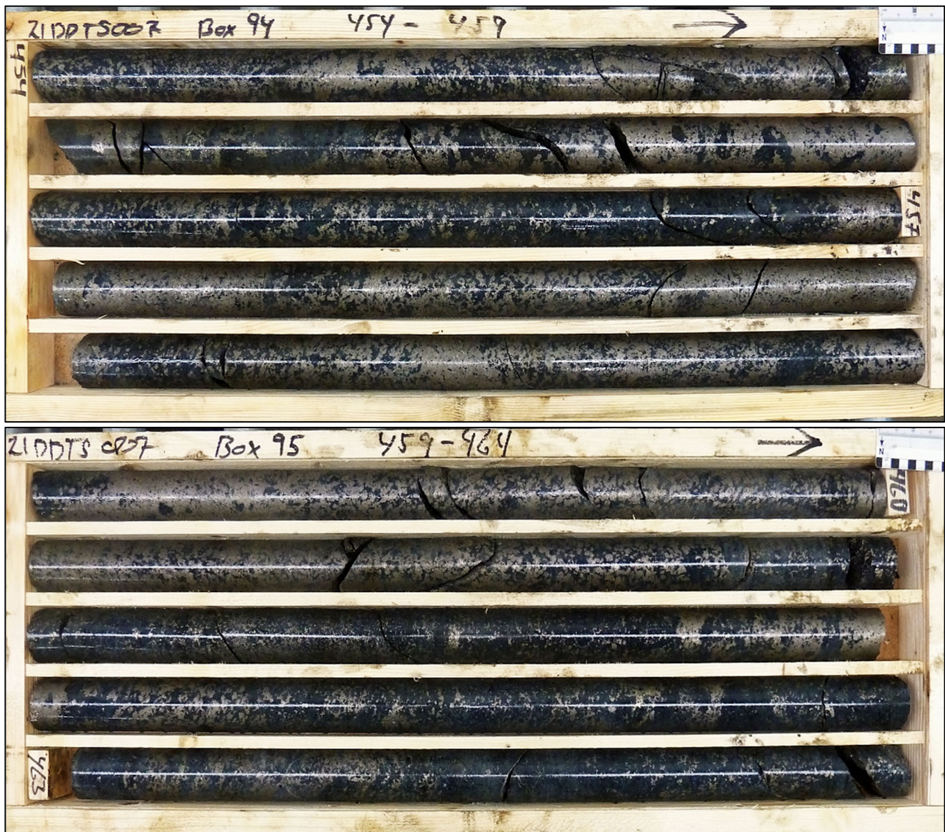
Figure 1: Magmatic Ni-Cu sulphides in 21DDTS007 displaying massive to semi-massive and matrix to coarse blebby sulphide mineralisation within the core of the host gabbroic intrusion (454m-464m shown)
