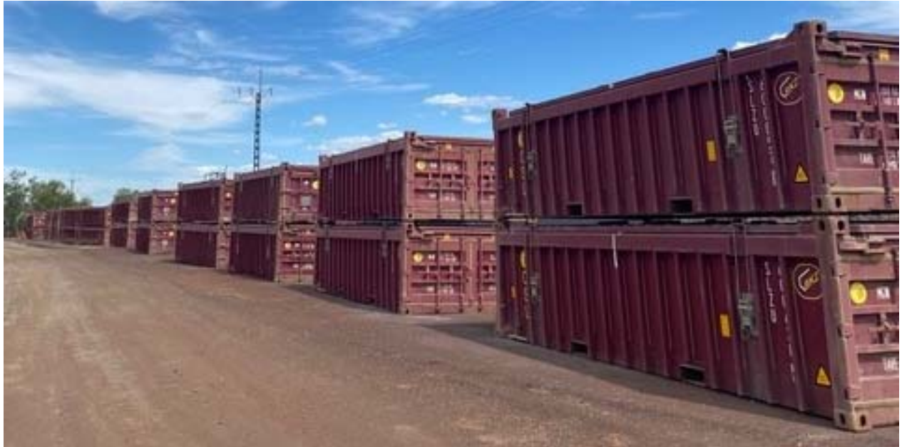
150 half height sea containers on-site ready to transport product to port (Product will be tipped out of containers into port shed and returned to site)
