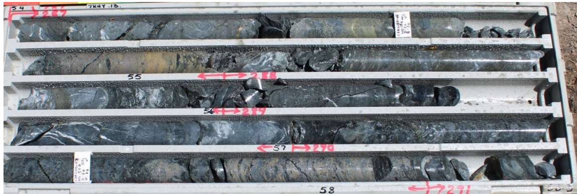
Figure 3 CRR21DD_08 at 54.45m depth. Close-up of banded pyrite – chalcopyrite sulphide mineralisation. Scale in centimetres, NQ core, 50mm diameter.
