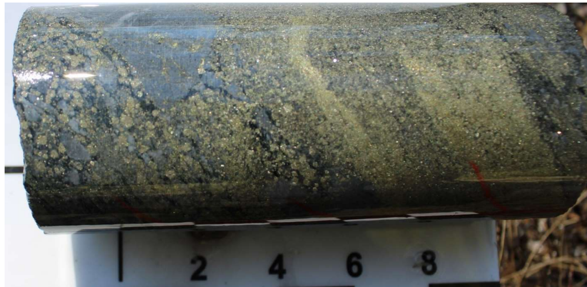
Figure 3 CRR21DD_08 at 54.45m depth. Close-up of banded pyrite – chalcopyrite sulphide mineralisation. Scale in centimetres, NQ core, 50mm diameter.
