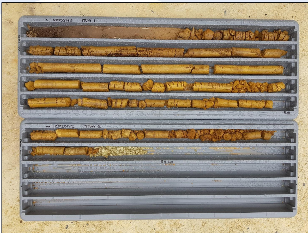
Figure 2 – Push Tube Core drillhole KMC0192 (Trial Pit)
