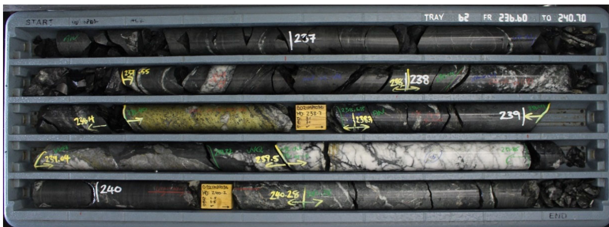
Figure 5: Steeply west dipping, Pyrite-Chalcopyrite-Quartz veining within DD21KP1036 with the Harbour View South main lode from 238.4m hosting 2.6m @ 1.23 g/t Au, 2.34 % Cu, 23.97 g/t Ag.
