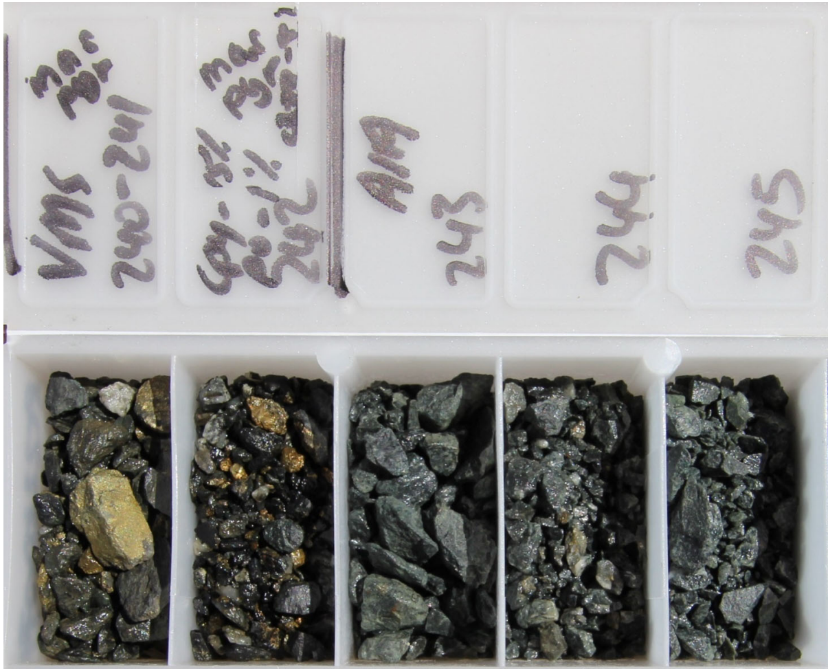
Figure 4: Massive sulphide (>80% sulphides) veining between 240m-242m comprised of pyrite (65%), chalcopyrite (15%), pyrrhotite (1%). The 2m interval from 240m graded at 7.7 g/t Au, 3.68 % Cu, 39.5 g/t Ag.
