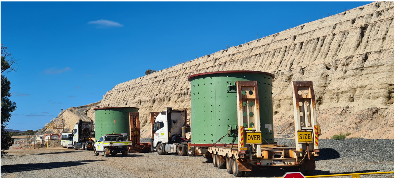
Ball Mill Shells being delivered.
