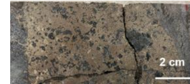
Massive sulphide in 20WGDD0005 (340.4 – 340.5m) grading 1.38% Ni
