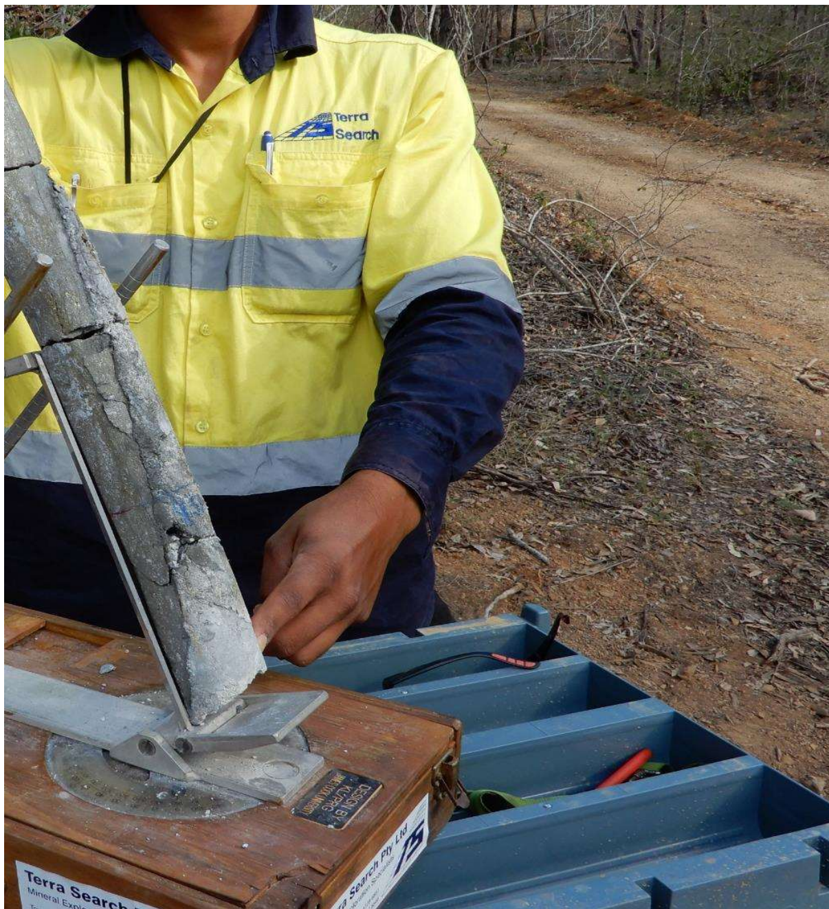
Fig 12. NQ Core Photo in Core Oriented frame CAE hole # 7, 451m showing sub vertical to steep west dipping fault quartz pyrite infill in sharp contact with rock crush zone/breccia . Massive pyrite with some quartz vein material infills the structure . View is looking south , orientation of contact is striking SE (140 magnetic). Interval 450m to 451m , 1m @ 81.64 g/t Au, 107.3 g/t Ag, 0.14 % Cu, 30.5 % S.
