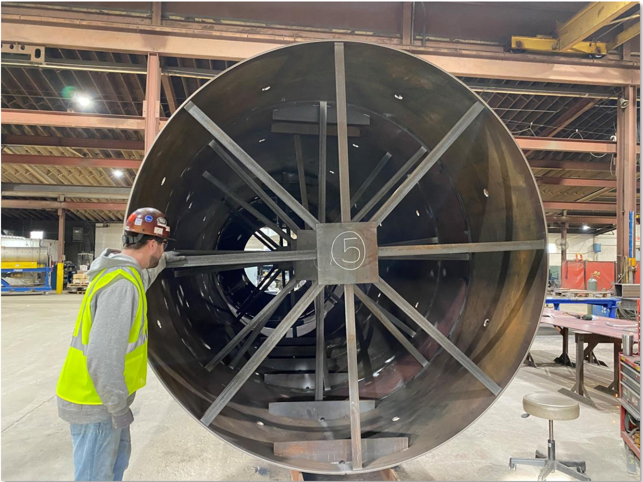
Figure 4 - FEECO Headquarters, Cabinda Phosphate Fertilizer Cooler Drum.
