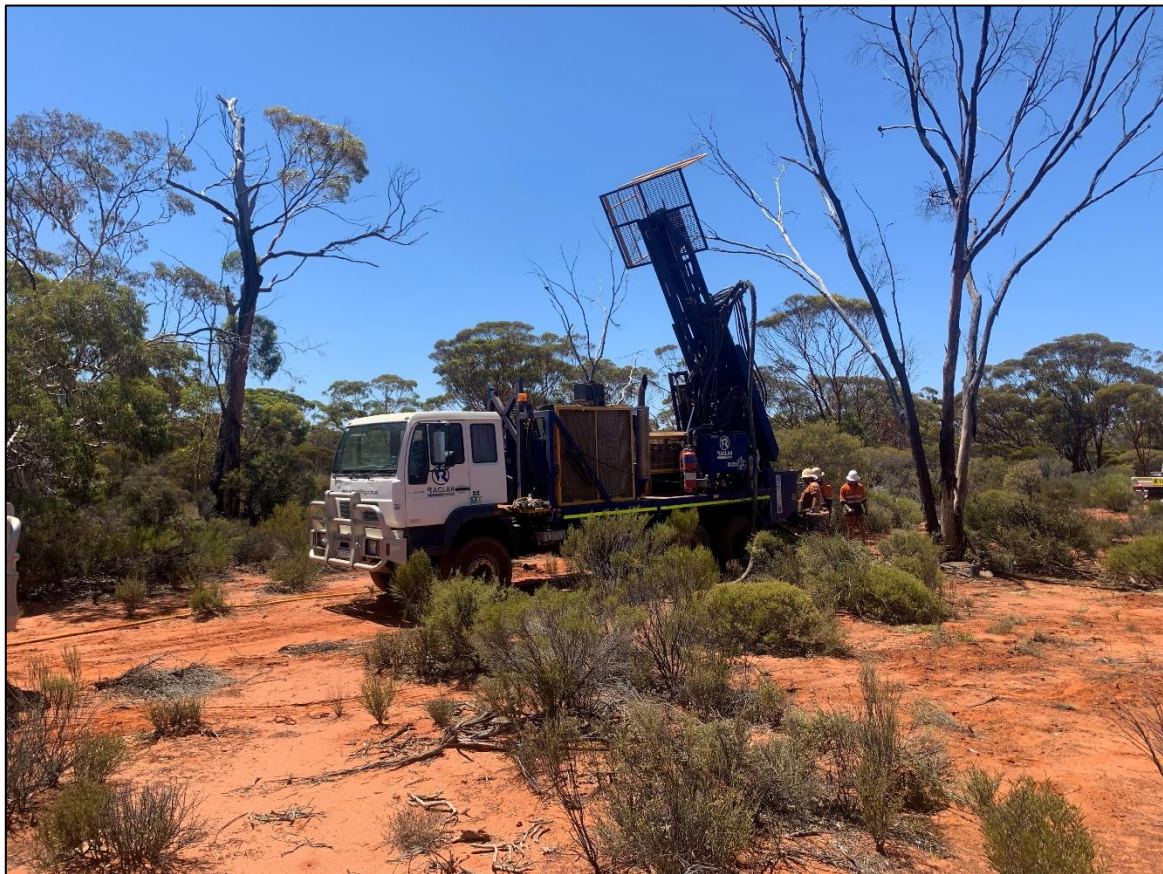
Figure 1 - Aircore drilling being completed at the Nepean Nickel Project.
