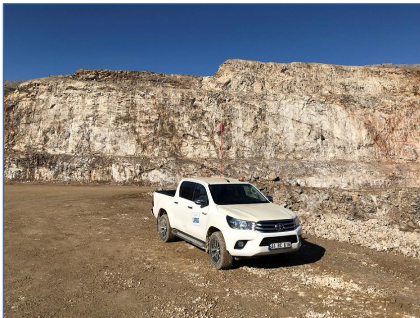
Figure 16.6 Typical 15 m Pre-Split at Çöpler Mine
