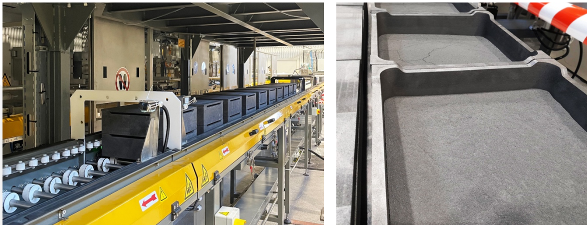
Figure 1 Part of EVA kiln during commissioning (L) and first batch of EVA Talnode ® -C (R)
