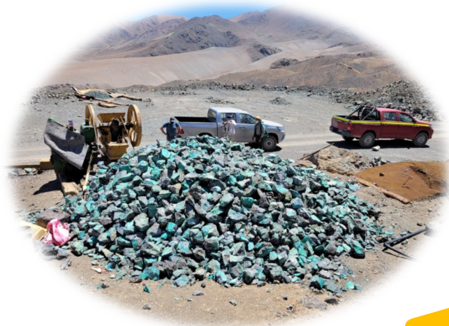
Stockpiled manto copper mineralisation from artisanal mining at Mostazal
