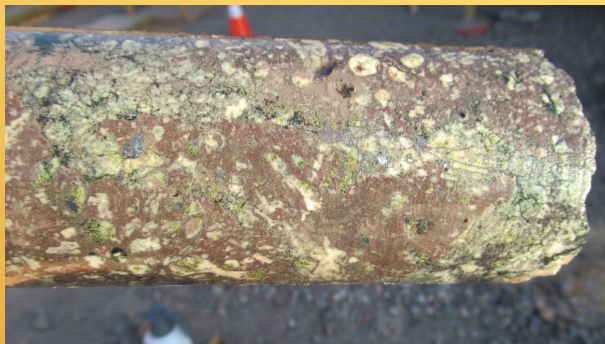
Altered andesitic basalt (MODD002) with fine grained disseminated pyrite, copper sulphides - chalcopyrite and bornite, and bornite amygdale fill*
