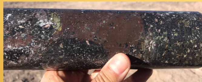
Altered porphyritic andesite host rock with disseminated and clotty sulphide mineralisation, including pyrite and chalcopyrite (copper sulphide) (MODD001)*
