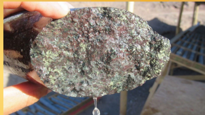
Altered andesitic basalt with fine grained disseminated pyrite and chalcopyrite (copper sulphide) (MODD002)*
