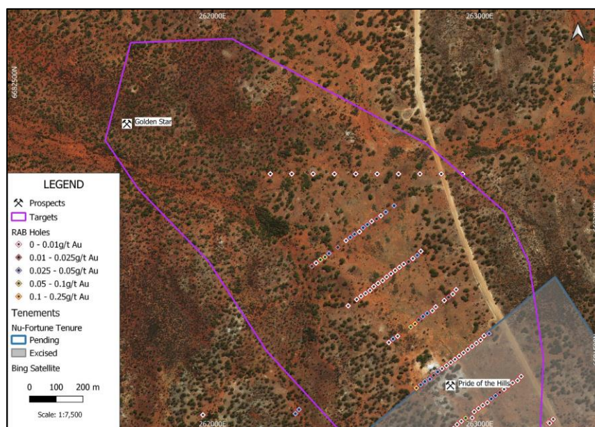
Figure 3:6 Mulwarrie E30/511 Sub-Project – Anomalous gold RAB intersections within Northern Extension Target area
