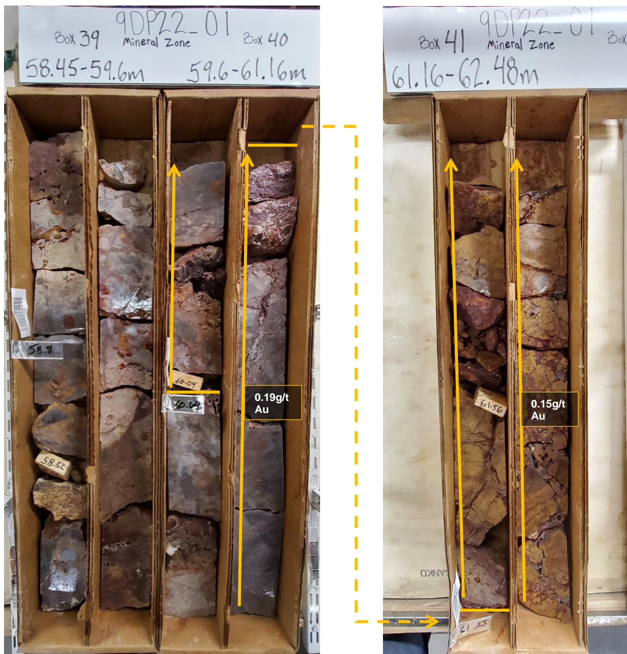
Figure 3: Photograph series of mineralised drill core from the hole 9DD22-001 with gold assays from 60.04 - 76.19m down hole. The overall mineralised intercept is 16.15m @ 1.04g/t Au which includes the internal waste intervals grading <0.15g/t Au.
