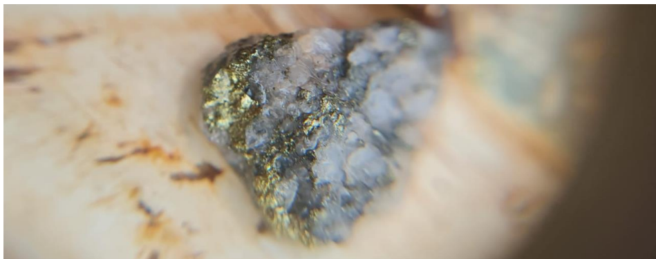
FIGURE 2: A BOTTOM-OF-HOLE CHIP FROM 21MBAC119 SHOWS CHALCOPYRITE-PYRITE MINERALISATION. COPPER ASSAYS ARE NOT YET AVAILABLE.
