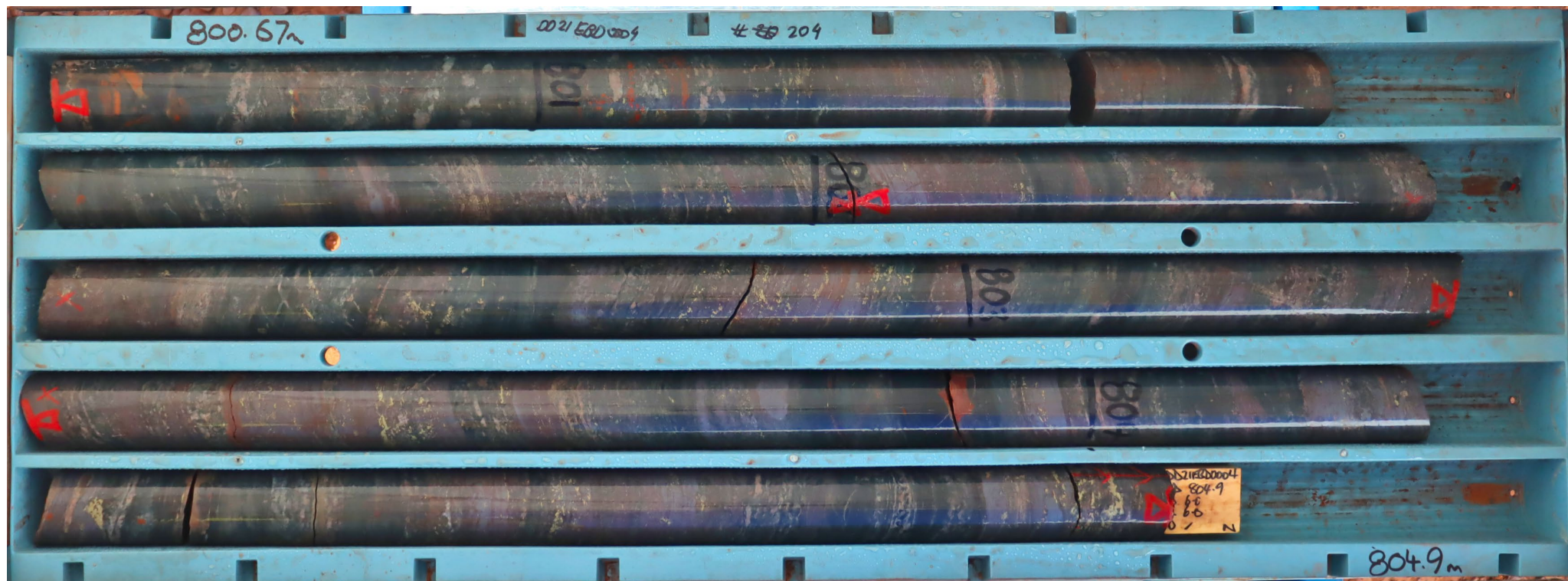
Figure 1 Mineralisation encountered in haematised Wallaroo Group sediments, drillhole DD21EBD0004. Dominated by chalcopyrite, the mineralisation consists principally of bedding aligned blebs and veinlets plus minor disseminations.
