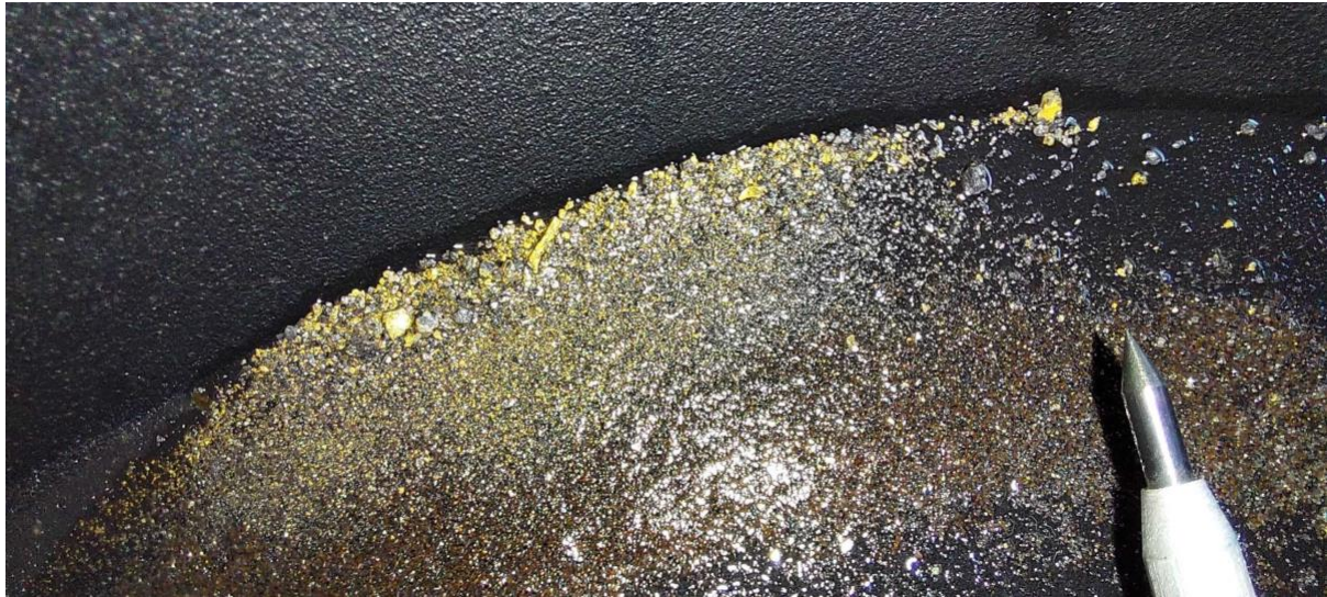
Photo 1: From a 360g sample split of drill hole 21MNRC007: 70 to 71 metres @ 190.06 g/t (Photon 500g assay), panned concentrates displaying coarse gold and sulphides in the tails. The metal scribe tip shown is 8mm long for approximate scale
