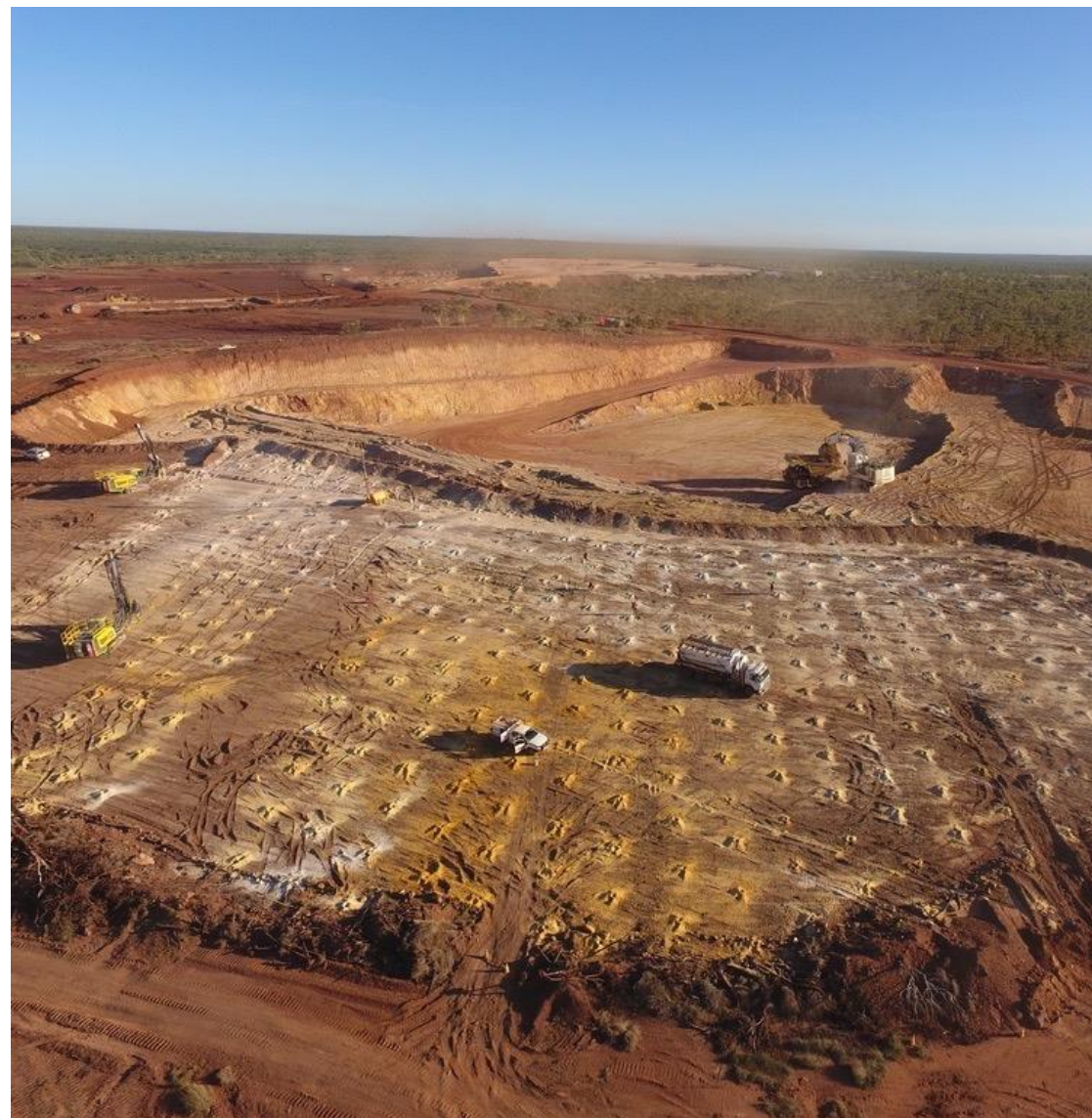
Mining at east pit 25 Feb22. Drilling and shot loading in the foreground and mining in centre. ROM pad in background with first ore stockpiled during February.
