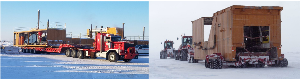
Figure 1: Mobilisation of Arctic Fox rig modules to Merlin-2 drilling location
