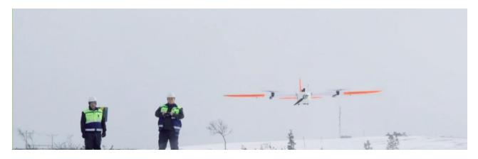
Figure 2. Drone equipment being utilized for the high-resolution magnetic survey.
