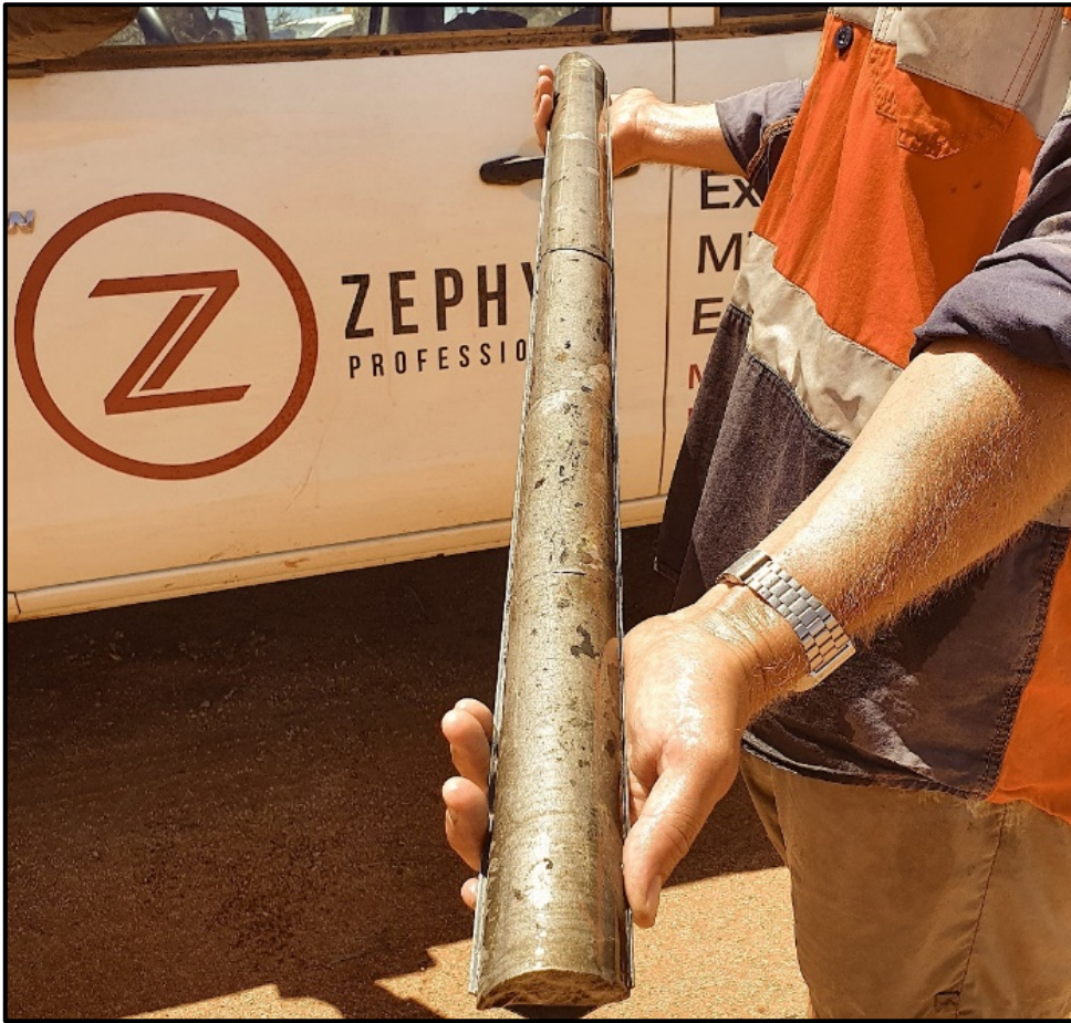
Figure 3: Photo of massive nickel sulphide in drill core of diamond hole TED07 at the Dusty Nickel Discovery– this part of the core grades 4.01% nickel (see text for details).
