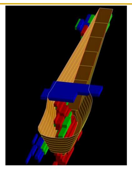
Figure 3: Approved Bulk Sample Pit design.
