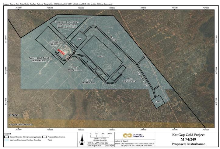
Figure 1: Bulk sample mining pit area (red) within Mining Proposal plan<sup>5</sup>
