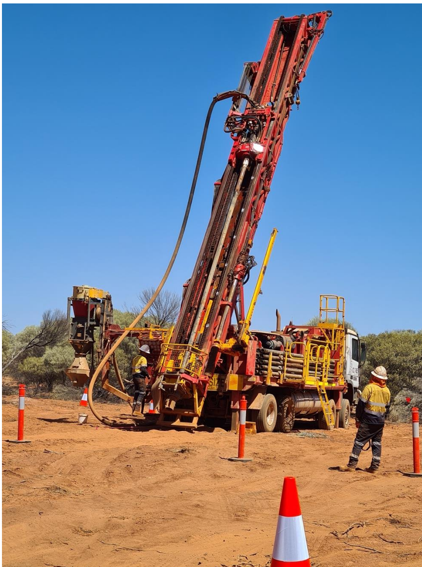
Figure 2: Drill rig in operation for Podium's Stage 9 RC drilling programme.
