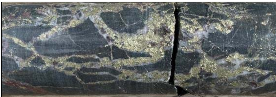
Photo 1. Chalcopyrite+quartz-filled fractures in chlorite+quartz-altered micro-diorite. 390.6m.
