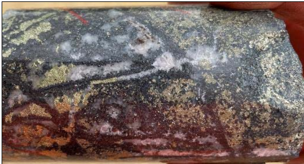
Photo 6. Semi-massive sulphide. Chalcopyrite+pyrite+quartz+hematite. Unusual texture of cross-cutting specular hematite and quartz veins. 416.1m.
