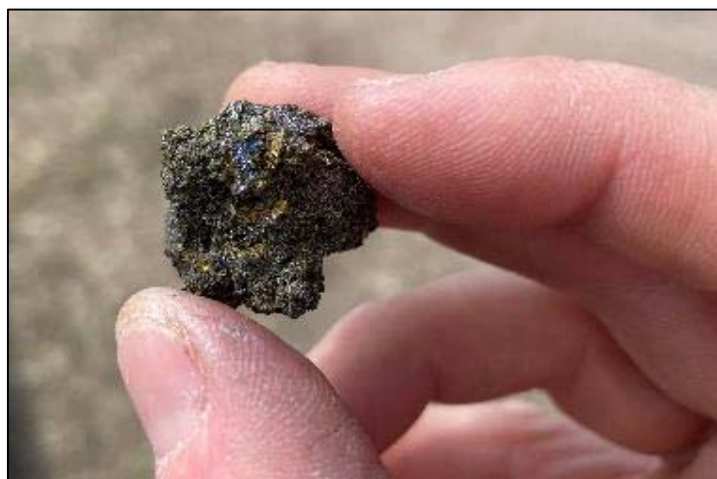
Photo 3. Massive chalcopyrite with bornite. 397.5m.
