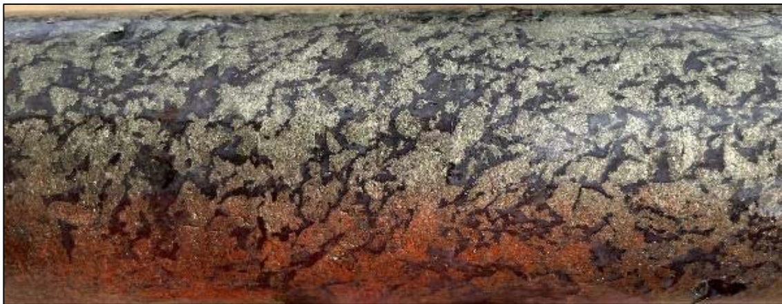
Photo 7. Massive chalcopyrite intergrowth with quartz+hematite gangue. 419.9m.
