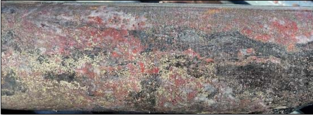
Photo 4. Semi-massive sulphide. Pyrite+chalcopyrite in hematite+quartz+chlorite rock. 399.0m.
