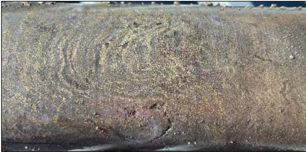
Photo 5. Massive pyrite with chalcopyrite bands. 399.9m.
