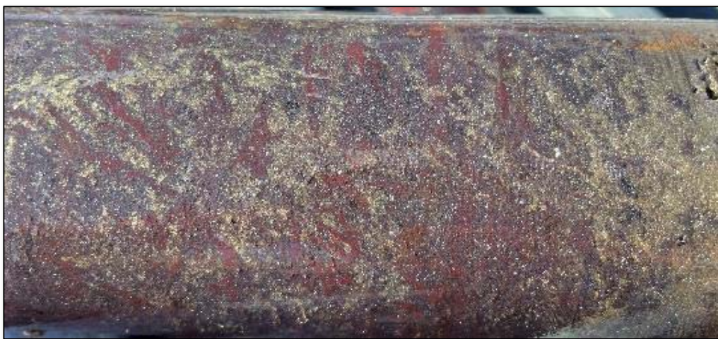
Photo 2. Semi-massive sulphide. Pyrite+chalcopyrite in hematite+quartz rock. 395.6m.
