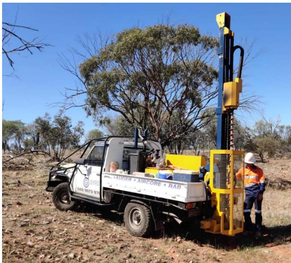
Figure 4. Gyro Drilling with 4WD Ute mounted auger rig
