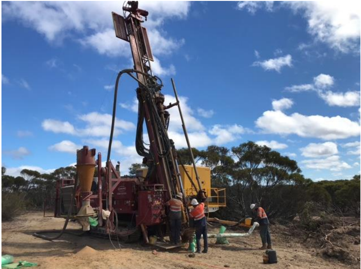
Figure 3: RC Drill Rig at RAV-4 West Deposit
