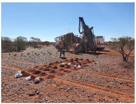
Figure 1 – Forrest Copper Project Air Core Drilling
