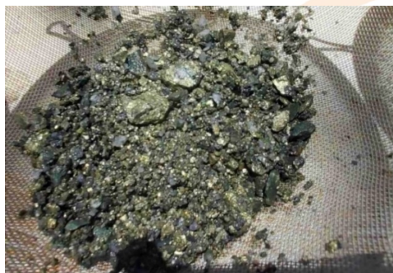
Figure 1. Sieve of sulphidic interval, 28-29m in HMLVRC014. Portable XRF analysis of 8.98% Cu upgraded by the lab analysis to 13.2% Cu and 3.2g/t Au.
