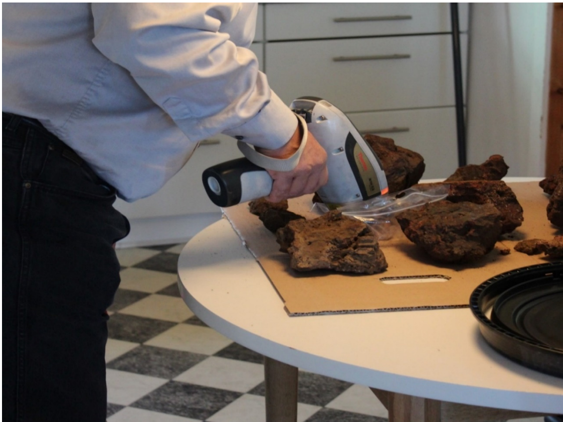
Figure 3. XRF testing large samples from Grønnedal-Ika
