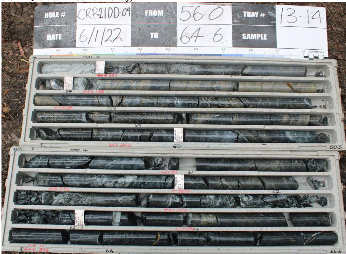
Figure 1 - Core showing mineralised interval from 56.2m – 59.8m (downhole), (Diamond drill hole CRRDD21_09, Scale: NQ core 50mm diameter variety)
