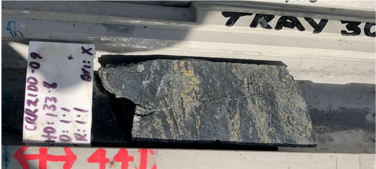
Figure 4 - Core from 133.8 – 133.9m (downhole) showing an interval of base metal sulphides with yellow-brown sphalerite (zinc) and lesser galena (lead) in black carbonaceous pelite. Interval 133.8-134.55m downhole assayed 3.87% Zn, 1.17%Pb, 0.21% Cu, 13.50g/t Ag, 0.03g/t Au. This mineralisation is part of a 10.05m downhole interval that extends from 131.05-141.1m downhole that comprises foliated black carbonaceous shale with disseminated and intermittent intervals (range from 1-10cm in width) of foliation parallel base metal sulphides (Diamond drill hole CRRDD21_09, Scale: NQ core 50mm diameter variety)
