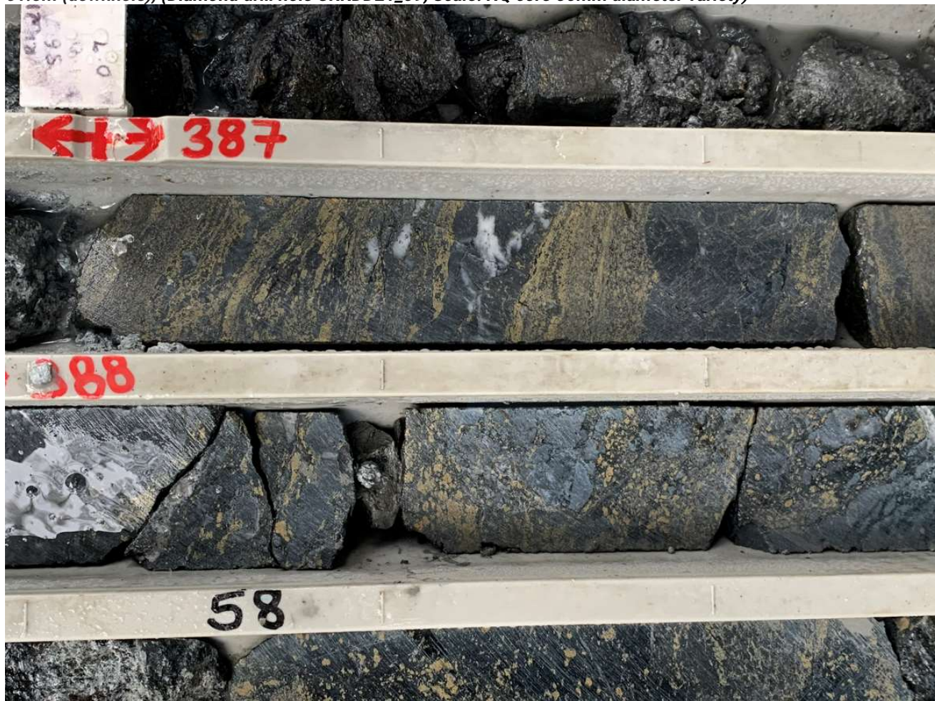
Figure 2 - Core showing a portion (56.2m – ~59m) of the mineralised interval from that extends 56.2m – 61.5m (downhole), (Diamond drill hole CRRDD21_09, Scale: NQ core 50mm diameter variety)
