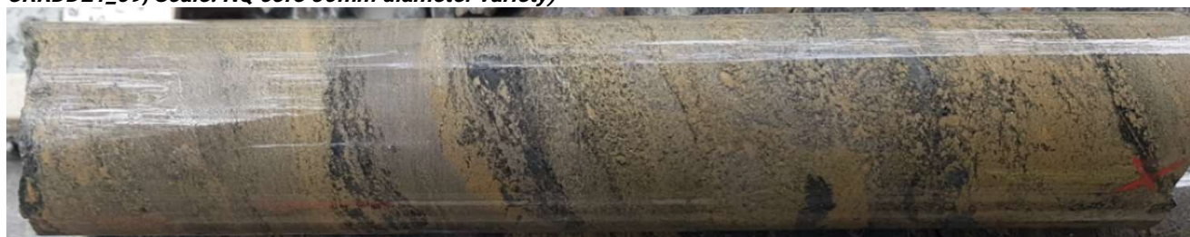
Figure 3 - Section of core from massive base metal sulphides that included 0.75 metres (57.05-57.8m) downhole that assayed 29.10% Zn, 12.15%Pb, 1.31% Cu, 51.60g/t Ag, 0.16g/t Au (Diamond drill hole CRRDD21_09, Scale: NQ core 50mm diameter variety)
